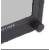
Pulse disc switch / ENTER switch on the cabin unit
